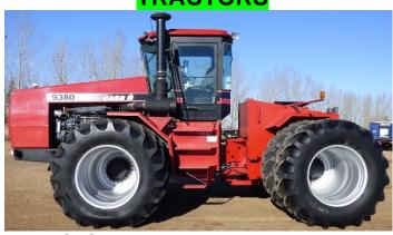
•1998 CASE IH 9380 4WD tractor, 3,382 hours, 400 hp. Cummins N14 engine, 710/70R38 duals. 12F/3R, 4 hyd's., Outback 360 GPS, exc. cond. •1995 CASE IH 9270 4WD tractor, 6,453 hours, 335 hp., 20.8R42 duals, 4 hyd's, 12F/3R., 1 owner.
