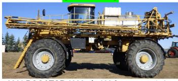
•2011 ROGATOR 1396 s/p 100 ft. sprayer, 1525 hours., 1,300 gal. ss tank, 20" spacing, autosteer, Raven Viper Pro monitor w/ Phoenix 200 receiver, 5 way nozzle body w/ Sharpshooter control, boom & height control + MANY MORE OPTIONS!
