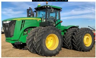
•2013 JOHN DEERE 9510R 4WD tractor, 3066 hours, 18 sp. powershift, 18F/6R, 510 hp 800/70R38 duals, weights, big 1000 pto., 5 high flow hyd's., Starfire 3000 GPS receiver, GS3 touchscreen, 7" color display, premium Command View II cab, power beyond hydraulic connectors, heated mirrors, HID lights, + MORE! •1978 CASE 1570 tractor, 4,936 orig. hours, 180 hp., 20.8 X 38 duals, 2 hyd's., powershift, 1000 pto., front weights, diff. lock, A/C.
