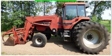
•1989 Case IH 7120 tractor w/ Case IH 710 FEL grapple, & 7 ft. bucket, 6,505 hours, 151 hp., 540/1000 pto., 18 speed full powershift transmission, 3 hyd's., 20.8 X 38 duals
