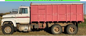
•1979 FORD 9000 t/a grain truck w/ 15.5 ft. wood box & hoist, roll tarp, 13 spd., manual transmission, 403,235 km showing, 2,108 hrs. showing, 365/80R20 fronts, 11R22.5 rears, 671 Detroit diesel, diff. lock, 66" high sides.
