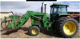
•1981 JOHN DEERE 4440 tractor w/ JD 260 FEL, grapple, & 7 ft. bucket, 8,417 hours, 130 hp., 540/1000 pto., power quad transmission, 3 hyd's., 18.4 – 38 duals, shedded.
