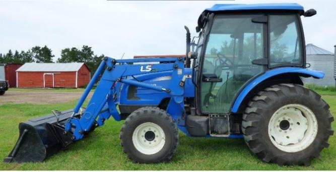
●2010 LS U5020 tractor w/ 6 ft. FEL & bucket, ONLY 420 hours, 47 hp., diesel, 3 pt. hitch, joystick, 540 pto., cab, A/C, syncro shuttle transmission, 17.5SL-24 rear tires, 12-16.5 fronts, shedded, excellent condition. S/N# 2136011933.
